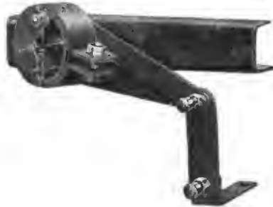
FOSTER SHOCK ABSORBER IN PLACE.
